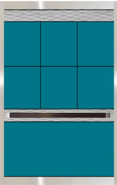
Artistic rendering. Actual design is proportionate to cab size. INTEFLEX™ BISTRO™ with Formica® Infinity 1520 laminate. Rigidized® 5WL® behind handrail and below the cap reveal. Black powder-coated panel reveals. Recessed stainless steel wall base, cap and wall reveal. Shown with 2" stainless steel flat bar handrail.
